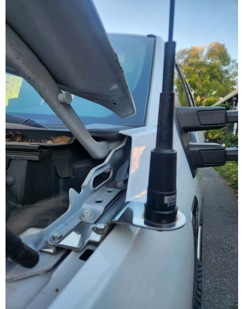
Dual band with mount designed for F250 hood
