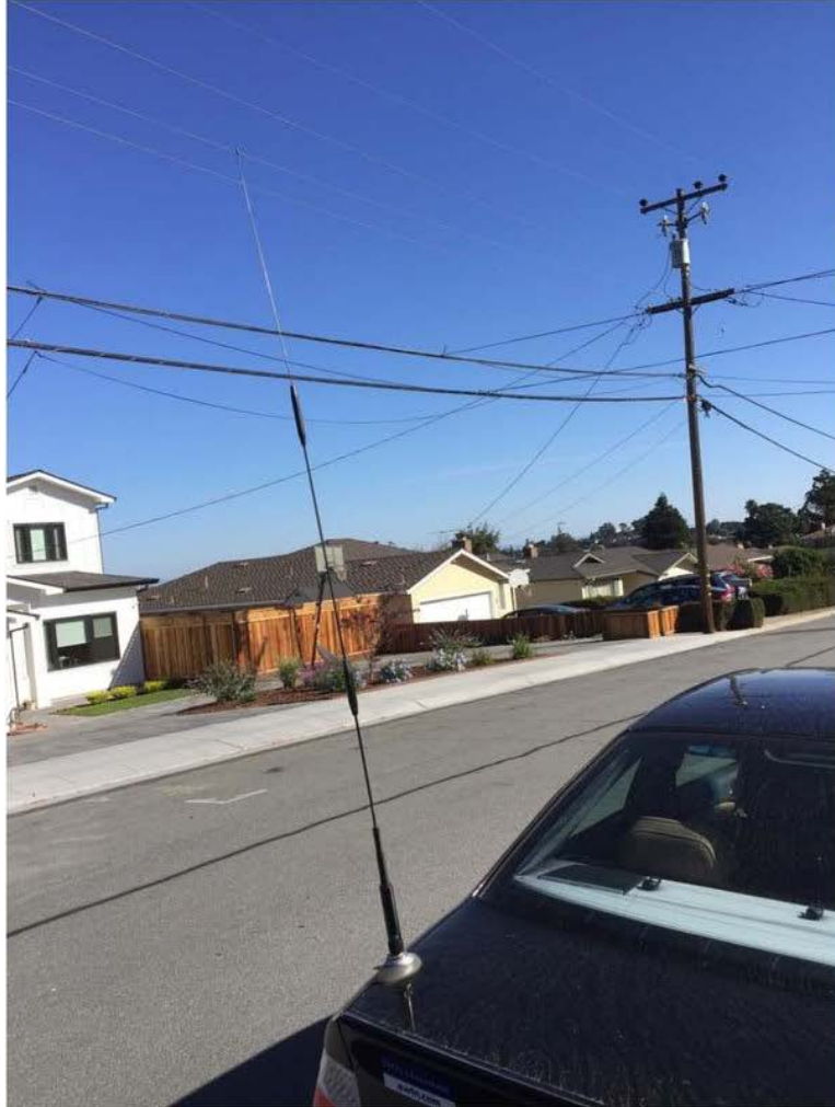
6/2/70 Antenna on mount, Note thin cable into trunk
